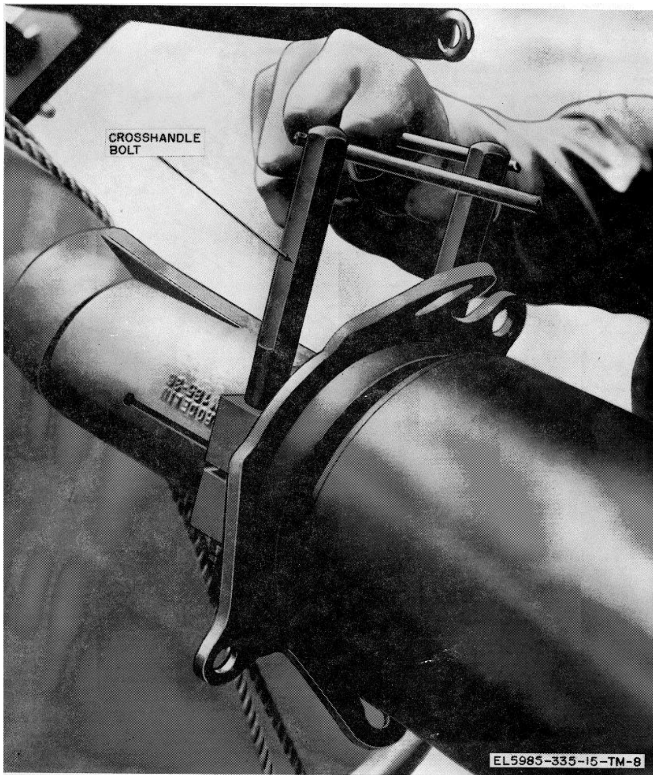
■ Figure 2-5. Tightening crosshandle bolts. (A)
